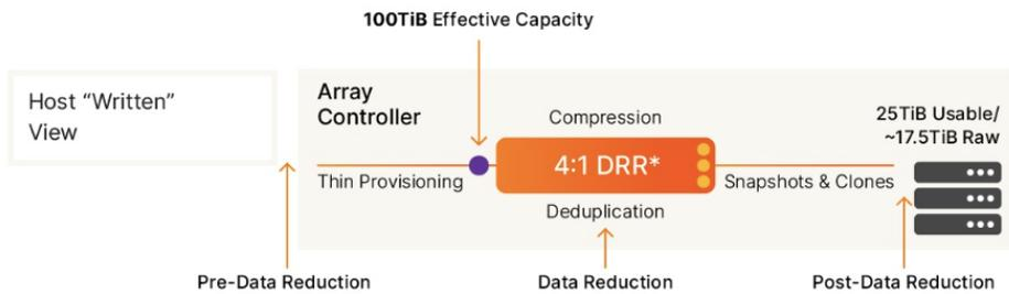
Figure 1. Block storage service effective used capacity example
